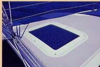
Built-in solar panel.
